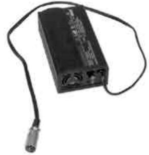
When the charger is plugged in, the orange "Charging" LED will illuminate. After charging is complete, the Charging LED will extinguish and the green "Charged" LED will light up. If both LED's are illuminated, the charger doesn't sense the presence of the batteries. Check for poor connections on batteries and you may wish to have batteries load tested or have charger checked out by your Dealer.
